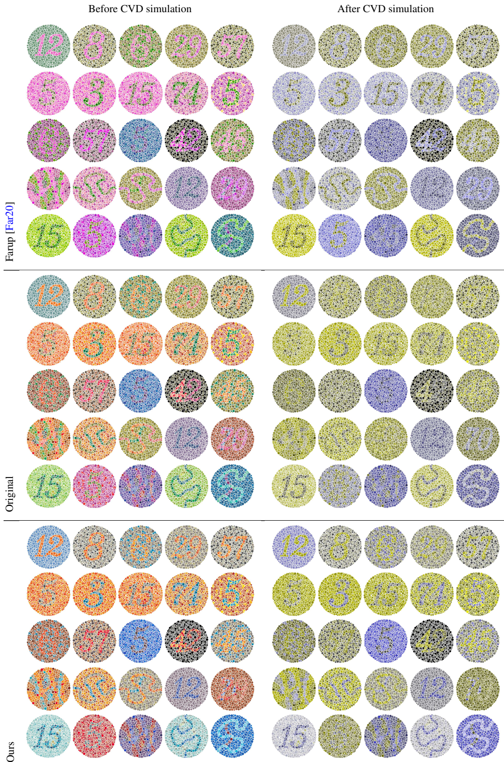
Figure 12: Results for a collection of Ishihara plates. The first two rows show benefits from daltonization, i.e., we can make out more numbers after simulation when daltonization is active. The middle plate in the middle row is an example where our algorithm is the only one successfully showing a number. We show worse results in the last plate on the next row, where no daltonization or Farup makes it easier to distinguish the number. On the last row, Farup’s method is the only one that clearly shows a 5 in the second plate, however, Farup also seems to indicate that the middle plate (bottom row) says 45, which the original image does not easily reveal. Simulated CVD: deuteranopia. Original image credit: Kaludov on VectorStock.com.
